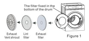
2. To properly clean your ventilation system, begin by removing the "exhaust vent shroud," "lint filter," and "exhaust filter." Taking care not to damage either filter, delicately remove any trapped lint or debris using a soft brush or a vacuum cleaner. Refer to figure 2 to ensure proper handling of the filters.
