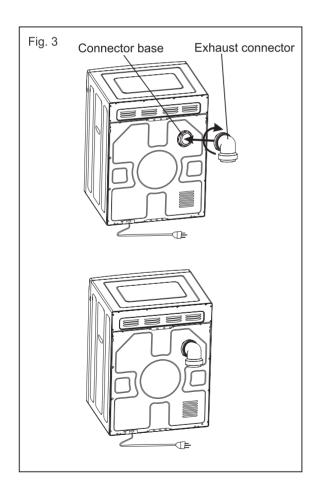
4. Rotate the Connector clockwise to fix the pipe to the Connector Base. Tighten.
