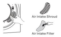
Slightly push upwards with your thumb until the latch hook disconnects, then remove.
